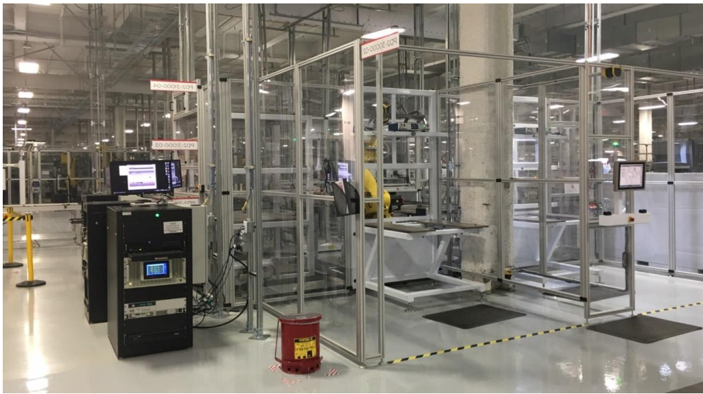
Figure 7-13 End of line testing showing emergency-off switches, bays with physical separation, and sensors for safety
