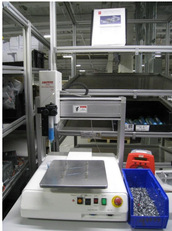
Figure 7-4 Automated application of thermal grease
