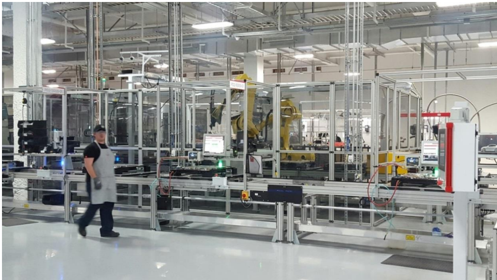
Figure 7-11 Pod line 2 Assembly and Testing - Robots are used for assembly automation and computerized testing with interlocks is done
