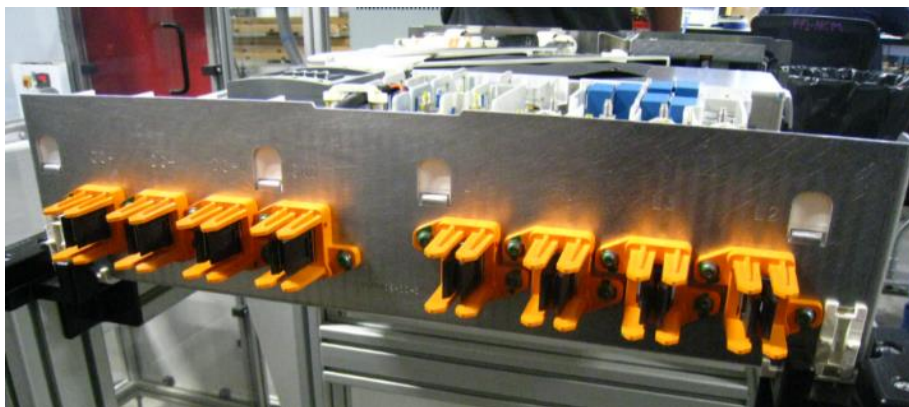
Figure 7-20 Blind-mate power connection
