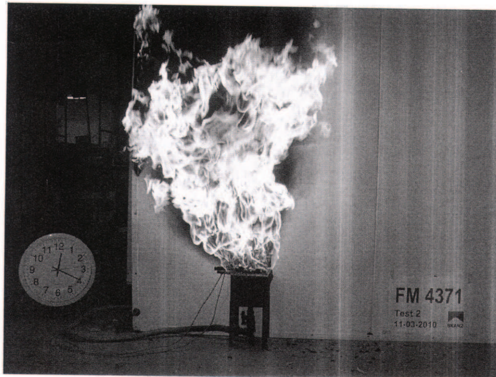
Figure 4 Wall test 2 – after 19 minutes (burner at 200 kW)
