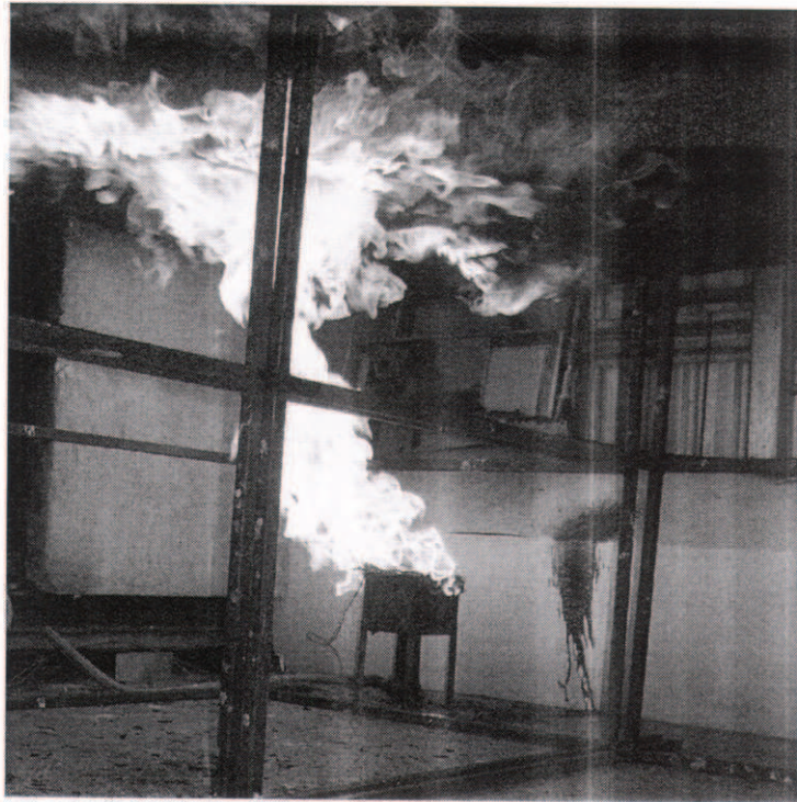
Figure 7 Ceiling test – after 21 minutes (burner at 300 kW)
