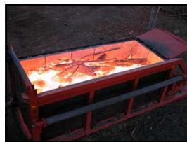
The curtain of air created in this process traps unburned fine particles under the curtain in the high temperature zone where temperatures can reach 1832° F (1000° C). The increased combustion time and turbulence results in a reburn and more complete combustion of the biomass.
