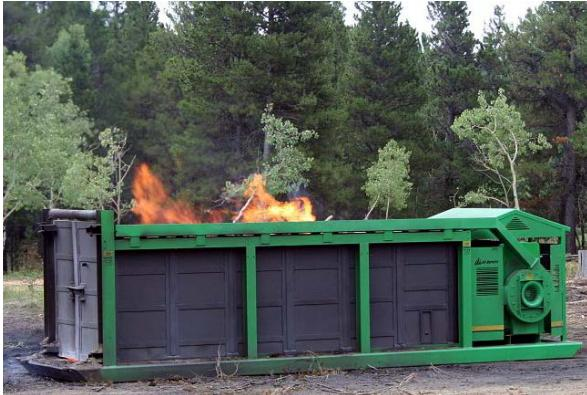
**General:** A self-contained, completely assembled above ground Air Curtain Burner (air curtain incinerator or FireBox) with a refractory lined burn-container for portable and permanent (stationary) applications. Designed for the high temperature burning of forest slash, land clearing debris, green waste, storm debris, and other waste streams in compliance with the requirements of US EPA 40CFR60.
