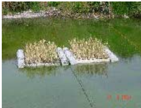
Newly planted vetiver on this floating platform. A trial is being conducted to determine the planting density needed to decontaminate this pond.
