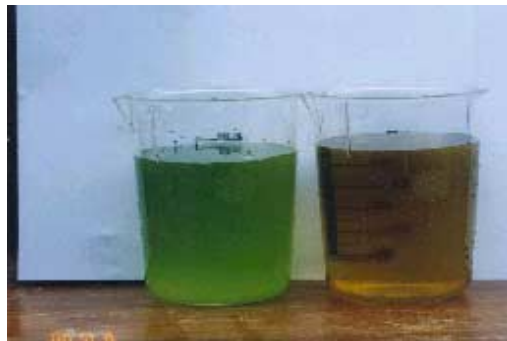
Left: Sewage effluent infested with Blue-Green algae due to high Nitrate (100mg/L) and high Phosphate (10mg/L) Right: Same effluent after 4 days treatment with vetiver, reducing N level to 6mg/L (94%) and P to 1mg/L (90%)
