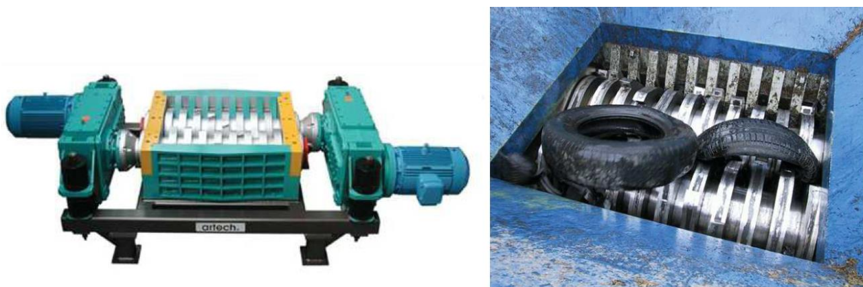
Figure 8 : Cisaille rotative mobile de type ARTECH RS 110/130
