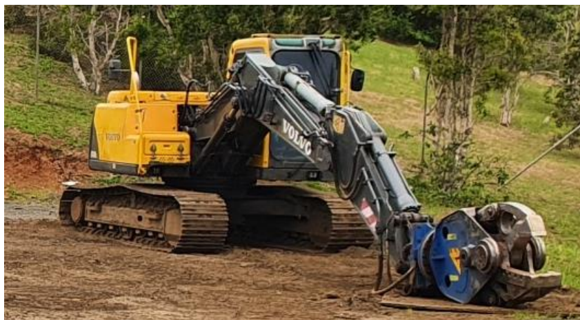
Figure 9 : Pelle hydraulique VOLVO 14 t, cisaille ARDEN
