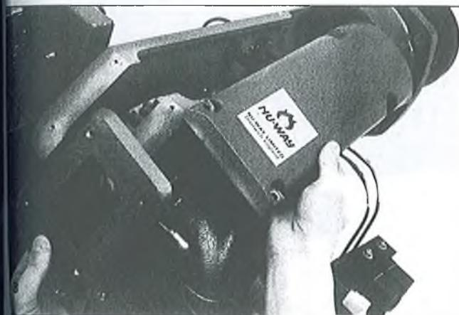
Remove top cover by undoing four screws. It may also be necessary to remove the four screws on the inspection window cover. To gain complete access to the fan it is advisable to remove the latter.
